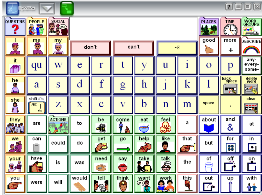
Picture Word Power is designed to allow access to over 100 core vocabulary items with a single hit. Linked page buttons are shaped as file folders. An onscreen keyboard includes word prediction.
