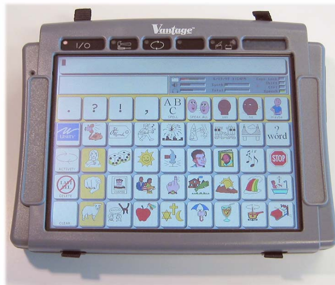
The Vantage provides access to a large vocabulary and displays Minspeak symbols.
